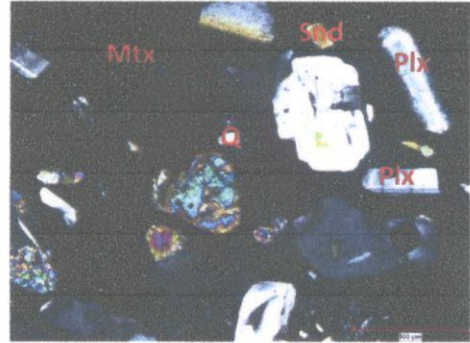
Şekil 1. Kayaç içerisindeki kuvars (Q), plajiyoklas (Plx), sanidine (Snd), hornblende (Hrb) mineralleri ve plajiyoklas mikrolitleri (Matriks) (Mtx-) (Çift nikol (sol - sağ). Figure 1. Quartz (Q), plagioclase (Plx), sanidine (Snd), hornblende (Hrb) minerals and plagioclase microlites (Matrix) (Mtx) were observed in rock (Crossed polarizers (left- right).
